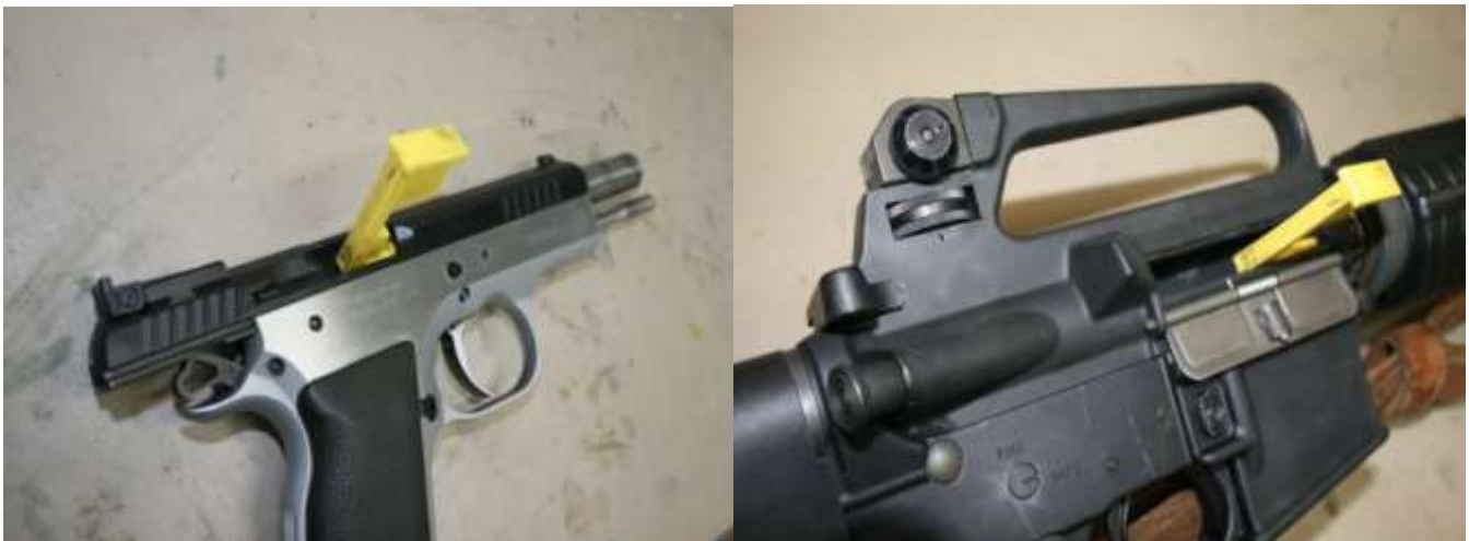
Figure 12. Examples of properly installed Empty Chamber Indicators
